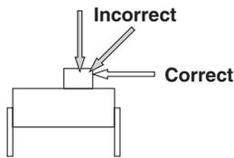
Set slide-type DIP Switches with a tiny, rounded object, such as the tip of a ball-point pen or a small screwdriver. Do not set the DIP Switch using tweezers or any other sharp object that may damage it. Do not set the DIP Switch using the point of a mechanical pencil, or lead powder or fragments may fall into the Switch and internal circuit board, causing the DIP Switch to malfunction and reducing the dielectric strength of the circuit board.
