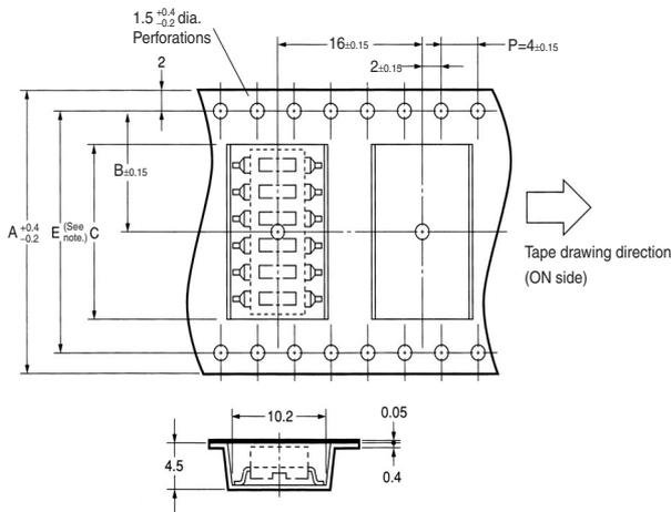
**Note:** The perforations along both sides are for Switches with 7 poles or more. The perforations on the bottom of the diagram are not provided on Switches with 6 poles or less.
