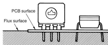
The A6S-H and A6H are designed specifically for reflow soldering. Do not use an automatic soldering bath or manual soldering for these models.
