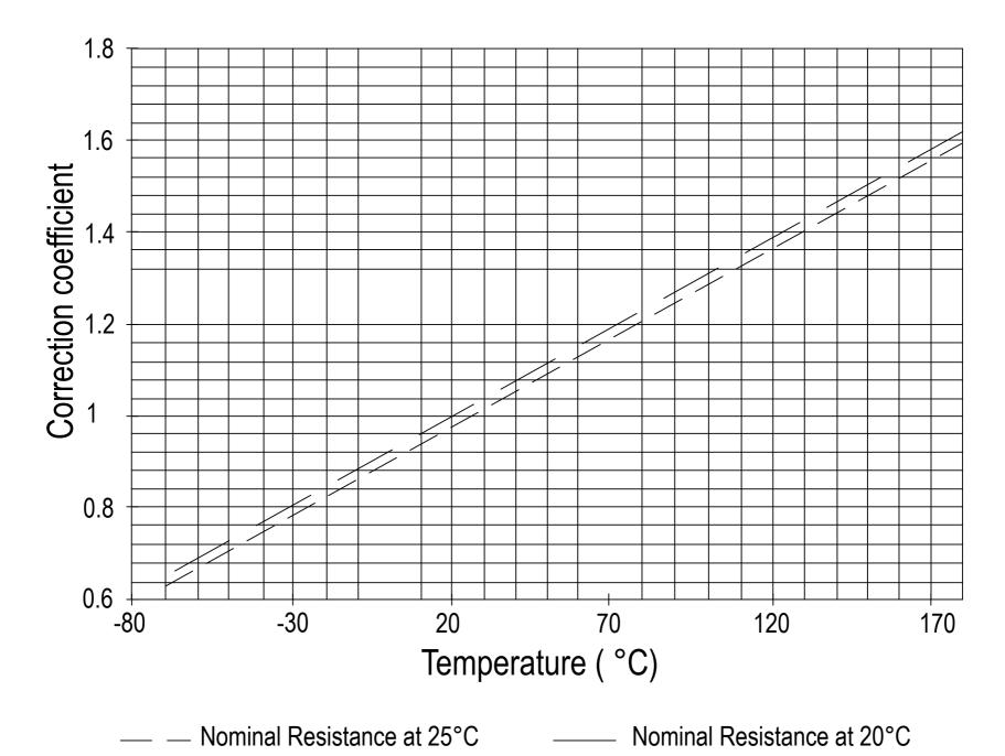
Example: Coil resistance at 25°C: 935 ohms. What is it at 125°C? Correction coefficient on diagram is: 1.39 at 125°C. R becomes: 935x1.39=1299 Ohms
