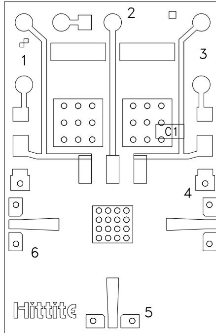
The grounded Co-Planar Wave Guide (CPWG) PCB input/output transitions allow use of Ground-Signal-Ground (GSG) probes for testing. Suggested probe pitch is 400mm (16 mils). Alternatively, the board can be mounted in a metal housing with 2.4 mm coaxial connectors.
