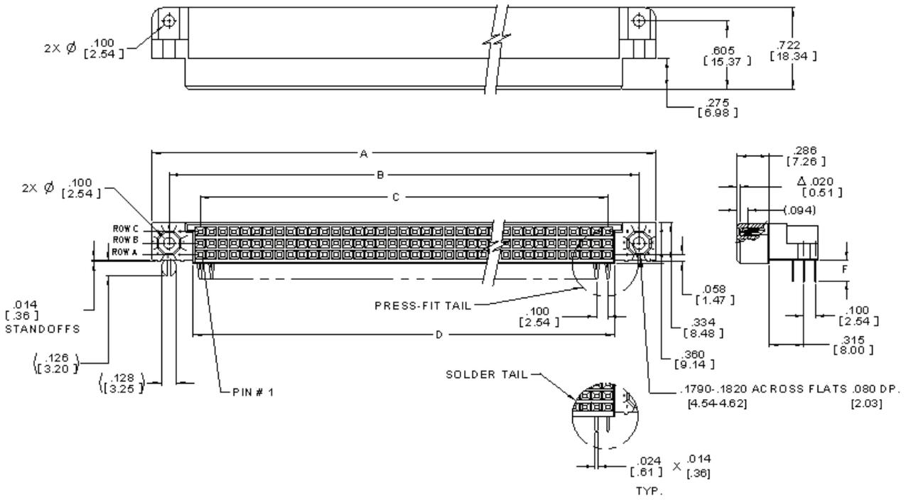
O 0.041- 0.049 PLATED-THRU HOLE, SOLDER TAIL
