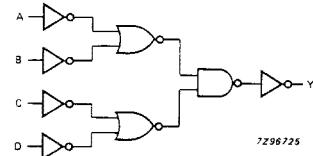
Fig. 5 Logic diagram (one gate).
