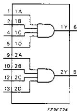
Fig. 4 Functional diagram.
