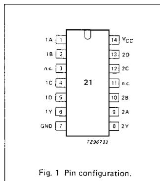
Fig. 1 Pin configuration.
