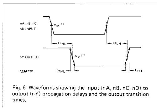
Fig. 6 Waveforms showing the input (nA, nB, nC, nD) to output (nY) propagation delays and the output transition times.
