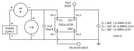
NOTE: A. CL includes probe and fixture capacitance. NOTE: B. An external .01µF bypass capacitor close to package ground and V<sub>CC</sub> pin is required
