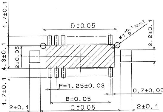
Note 1.If the pattern exists in the shaded area, and isn't treated with resist, it could touch the connector contact.
