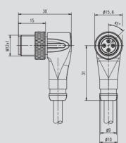
Contacts Cable jacket Order No. З PVC C112 10B013\_ 10 PUR C112 10B043 10 4 PVC C112 10B024 10 PUR C112 10B054 10 5 PVC C112 10B035 10 PUR C112 10B065 10
