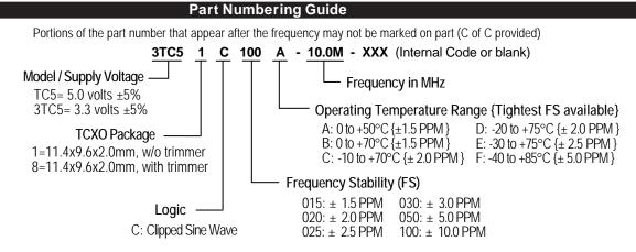
Consult factory for available frequencies and specs. Not all options available for all frequencies. A special part number may be assigned. Frequency Stability is inclusive of frequency shifts due to calibration, temperature, supply voltage, shock, vibration and load
