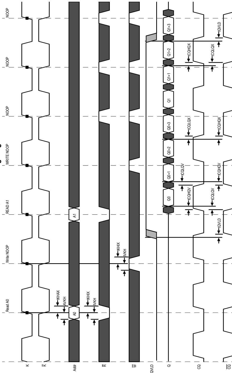
Read-Write CQ-Based Timing Diagram
