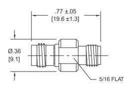
Note: Dimensions in Brackets are Expressed in Millimeters and are for Reference Only.
