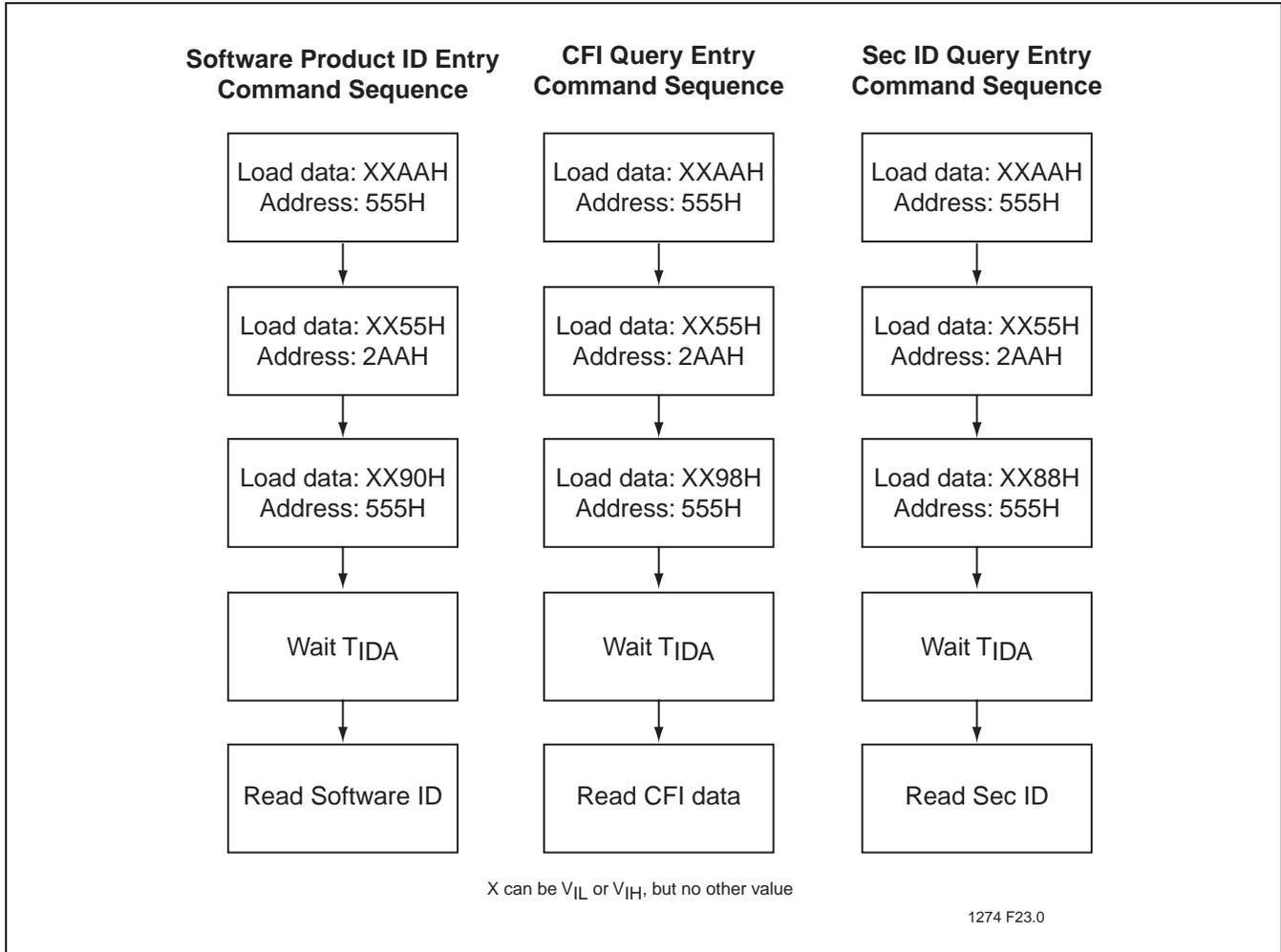
FIGURE 25: SOFTWARE PRODUCT ID/CFI/SEC ID ENTRY COMMAND FLOWCHARTS
