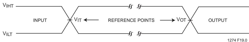
AC test inputs are driven at  $V_{IHT}$  ( $0.9 V_{DD}$ ) for a logic "1" and  $V_{ILT}$  ( $0.1 V_{DD}$ ) for a logic "0". Measurement reference points for inputs and outputs are  $V_{IT}$  ( $0.5 V_{DD}$ ) and  $V_{OT}$  ( $0.5 V_{DD}$ ). Input rise and fall times (10%  $\leftrightarrow$  90%) are  $<5$  ns.
