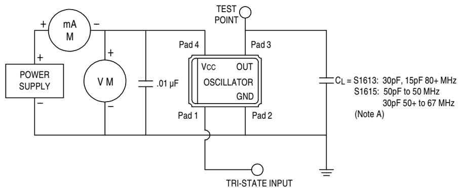
Note A:  $C_L$  includes probe and jig capacitance.
