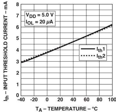
Figure 2. Typical input threshold current vs. temperature.
