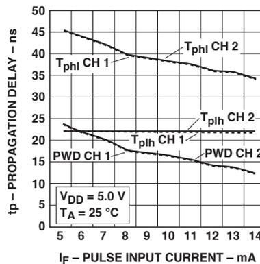
Figure 5. Typical switching speed vs. pulse input current.
