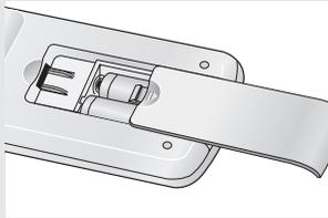
◀ Make sure to match the “+” and “-” ends of the batteries with the diagram inside the compartment.
