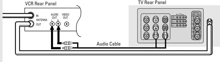
Make sure the jacks you are using are underneath the number “2.”
