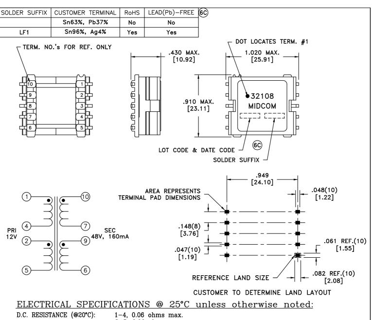
2-5, 0.06 ohms max. 6-9, 1.20 ohms max. 7-10, 1.20 ohms max.
