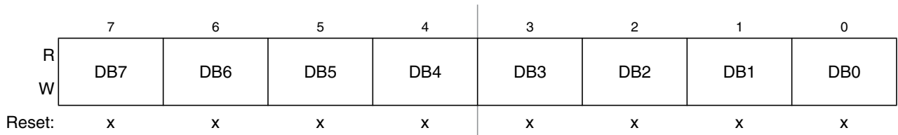
Figure 10-33. Data Segment Registers (DSR0–DSR7) — Extended Identifier Mapping
