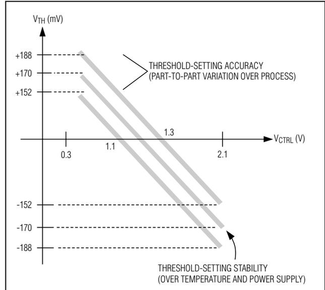
Figure 2. Relationship Between Control Voltage and Threshold Voltage
