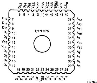
**Figure 1. Programming Pinout**
