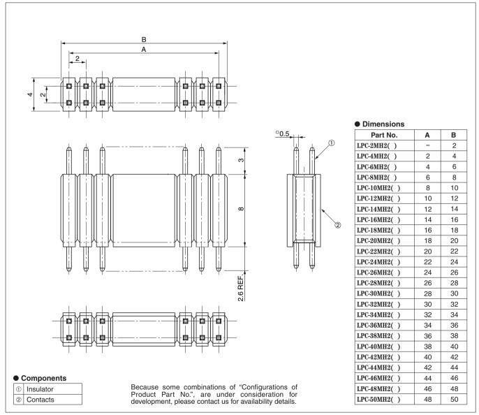
Mating connectors: LPC series female connectors or shunt plugs
