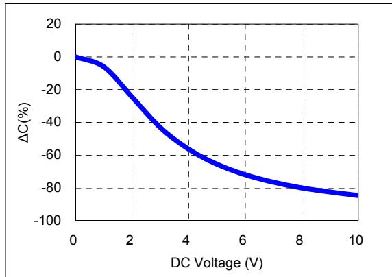
4) Bias TCC characteristics (Agilent 4284A, 1kHz, 0.5Vrms, 5Vdc)
