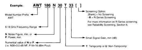
This example would order a 6–18 GHz amplifier with a noise figure of 3.0 dB max, temp comp, a small signal gain of 33 dB minimum, and NO "R" Series Screening.
