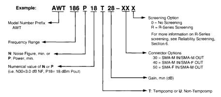
This example with a –40R suffix would order a 6–18 GHz amplifier with a Pout of 18 dBm minimum, temp comp, a small signal gain of 28 dB minimum, a SMA-male input connector and SMA-female output connector, and "R" Series Screening.
