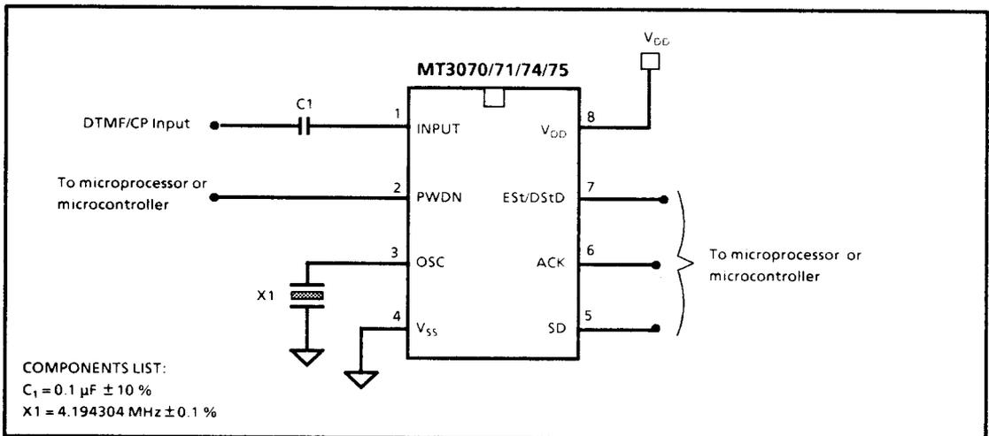
Figure 4 - Application Circuit
