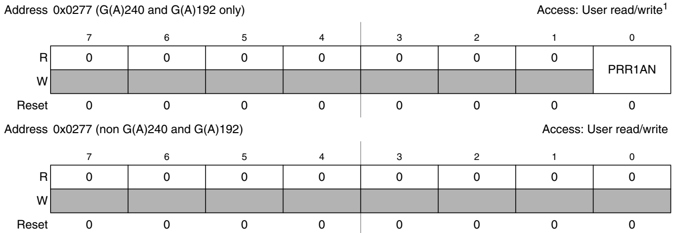
Figure 2-55. Pin Routing Register (PRR1)
