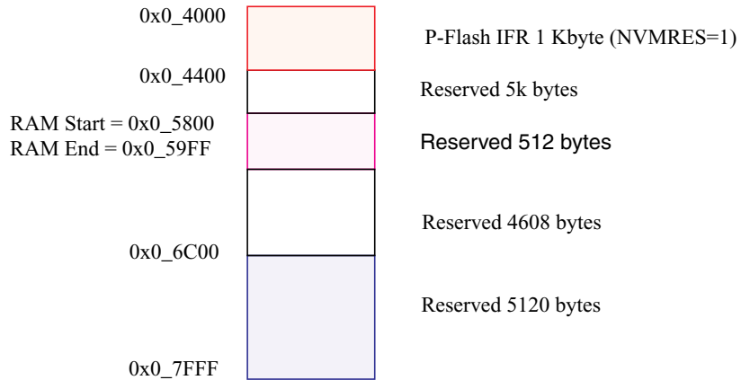
Figure 24-3. Memory Controller Resource Memory Map (NVMRES=1)
