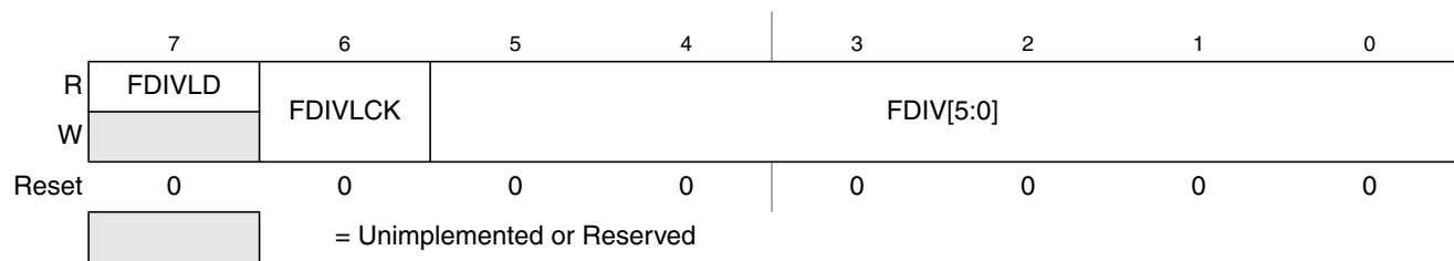
Figure 27-5. Flash Clock Divider Register (FCLKDIV)
