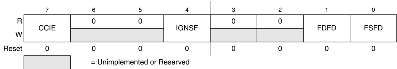
Figure 27-9. Flash Configuration Register (FCNFG)
