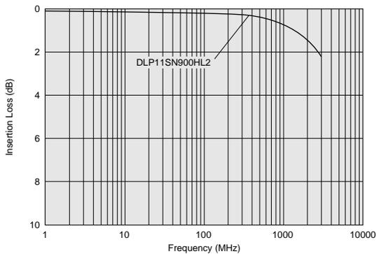
**Differential Mode Transmission Characteristics (Typ.)**
