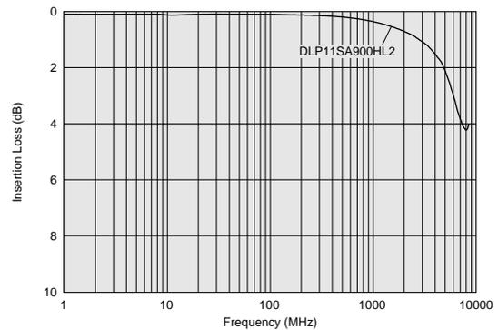
**Differential Mode Transmission Characteristics (Typ.)**
