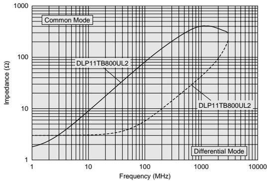
**Differential Mode Transmission Characteristics (Typ.)**
