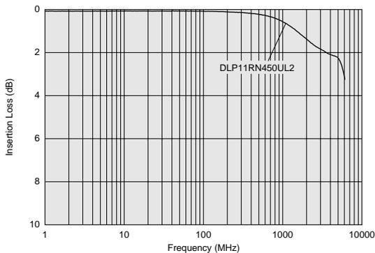
**Differential Mode Transmission Characteristics (Typ.)**
