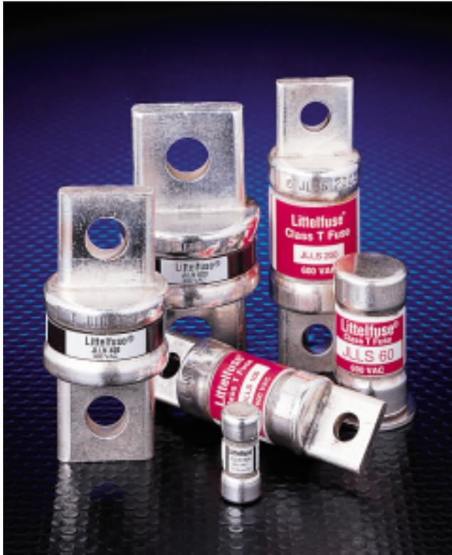
Space saving POWR-T™ fuses are the most compact fuses available in ratings above 30 amperes — less than one-third the size of comparable Class R fuses. When rated in accordance with the NEC, POWR-T fuses provide fast-acting overload and short circuit protection for non-inductive circuits and equipment. Used in inductive circuits, the ampere rating of POWR-T fuses must be increased to prevent opening on inrush currents. In such instances, POWR-T fuses may provide only short circuit protection.
