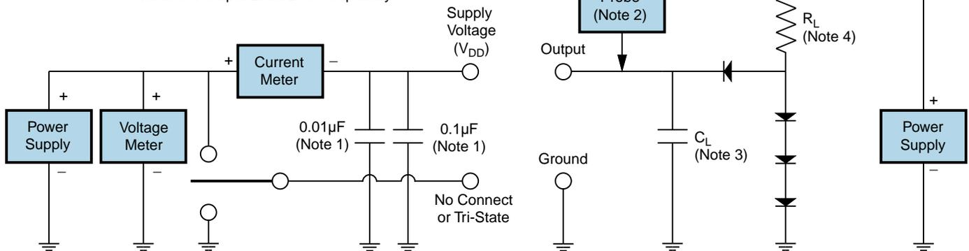
Note 1: An external 0.1 $\mu$ F low frequency tantalum bypass capacitor in parallel with a 0.01 $\mu$ F high frequency ceramic bypass capacitor close to the package ground and  $V_{DD}$  pin is required.
