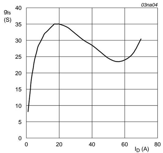
$T_j = 25^\circ\text{C}; V_{DS} = 25\text{V}$
