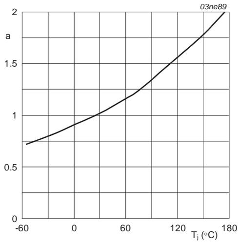
$$a = \frac{R_{DSon}}{R_{DSon(25^{\circ}C)}}$$
