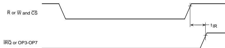
Figure A-6. Interrupt Reset Timing
