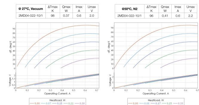
**Note**: Performance data is specified for optimal optimal conditions (TEC hot side is stabilized at ambient temperature). Heatsink thermal resistance is not included into estimations. Use TECCad Software for estimations under different conditions.
