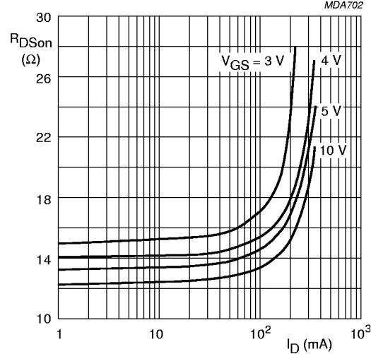
Fig.7 Typical on-resistance as a function of
