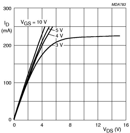
Fig.5 Typical output characteristics; T<sub>j</sub> = 25 °C.
