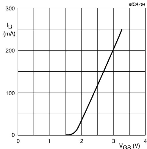
Fig.6 Typical transfer characteristic;
