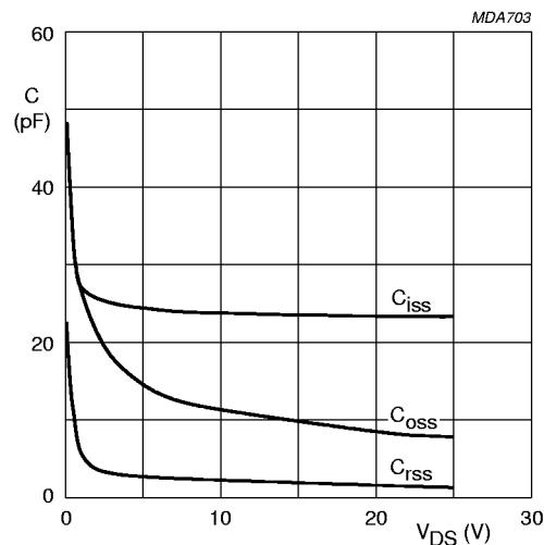
Fig.8 Typical capacitances as a function of
