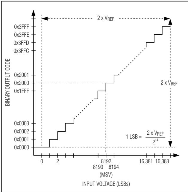
Figure 11. 0 to +5V Unipolar Transfer Function
