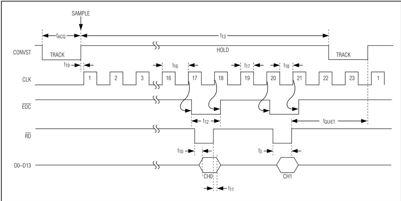
Figure 6. Read During Conversion—Two Channels Selected, External Clock
