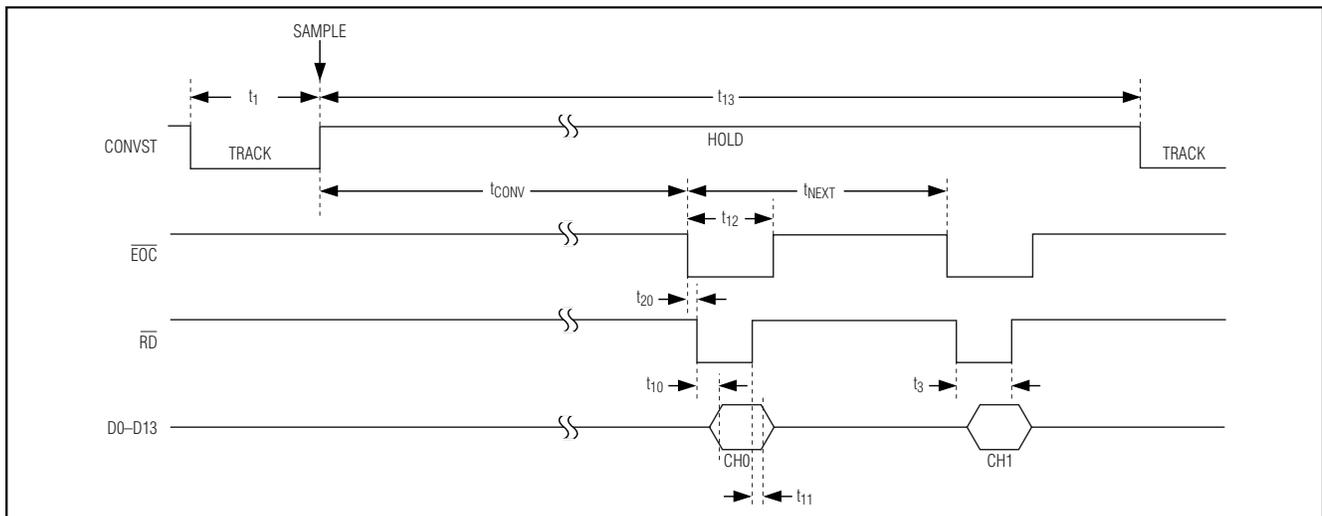
Figure 5. Read During Conversion—Two Channels Selected, Internal Clock
