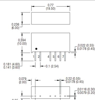
All dimensions in inches  $\pm 0.01$ (mm $\pm 0.25$ mm). All pins on a 0.1(2.54) pitch and within  $\pm 0.01$ (0.25) of true position.
