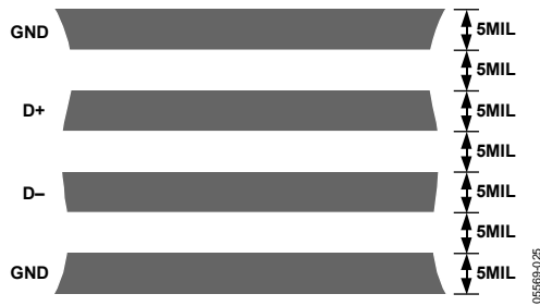
Figure 35. Typical Arrangement of Signal Tracks
