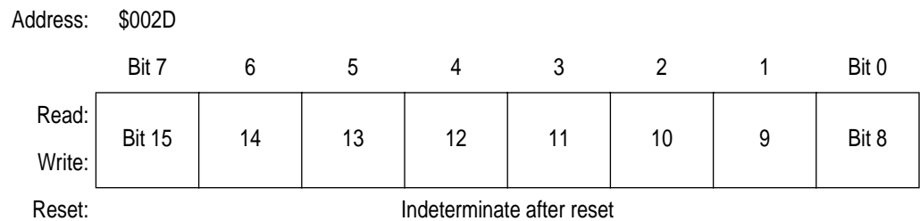
Figure 11-18. TIMA Channel 2 Register High (TACH2H)
