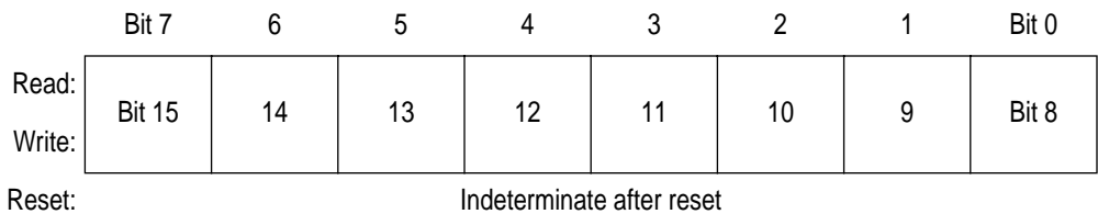
Figure 12-18. TIMB Channel 2 Register High (TBCH2H)
