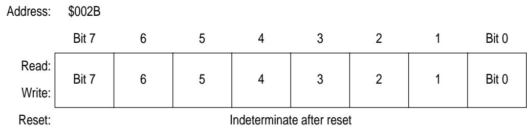
Figure 11-17. TIMA Channel 1 Register Low (TACH1L)
