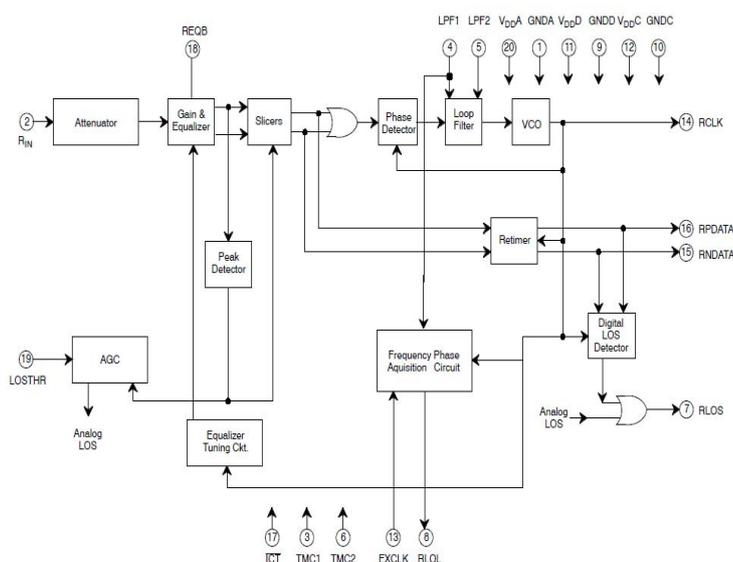
Figure 1. Block Diagram
