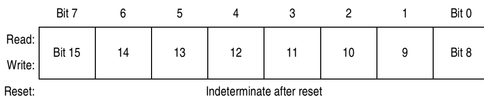
Figure 22-12. TIM Channel 0 Register High (TCH0H)
