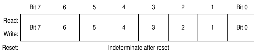
Figure 22-13. TIM Channel 0 Register Low (TCH0L)
