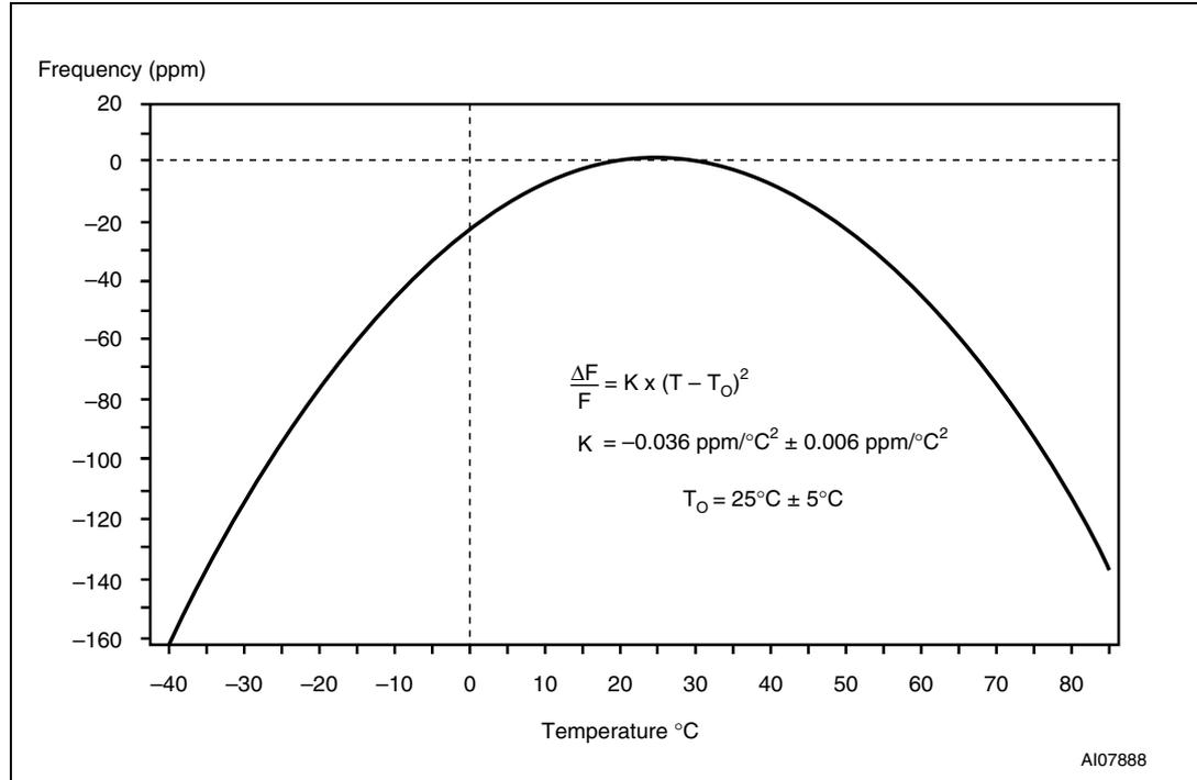
**Figure 11. Clock calibration**
