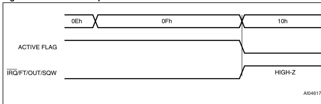
**Figure 13. Back-up mode alarm waveform**
