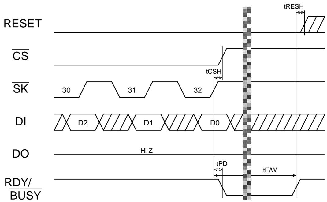
WRITE Ready /  $\overline{Busy}$  Signal Output ( $\overline{RDY}/\overline{BUSY}$  pin)
