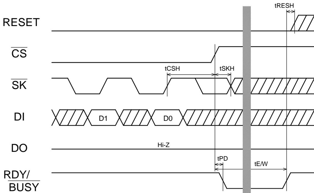
PAGE WRITE Ready /  $\overline{\text{Busy}}$  Signal Output ( $\text{RDY}/\overline{\text{BUSY}}$  pin)
