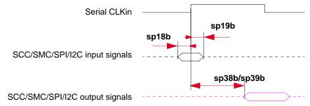
Figure 4. SCC/SMC/SPI/I<sup>2</sup>C External Clock Diagram
