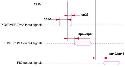
Figure 6. PIO, Timer, and DMA Signal Diagram
