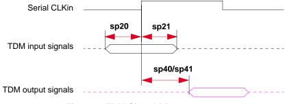
Figure 7. TDM Signal Diagram
