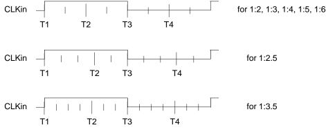
Figure 11. Internal Tick Spacing for Memory Controller Signals
