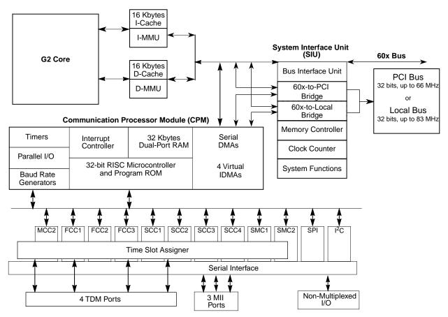
Figure 1. MPC8250 Block Diagram
