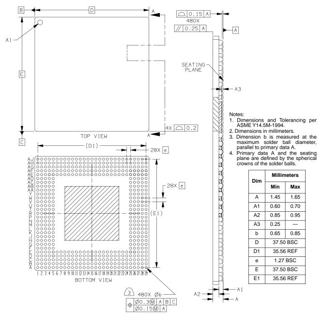
Figure 14. Mechanical Dimensions and Bottom Surface Nomenclature
