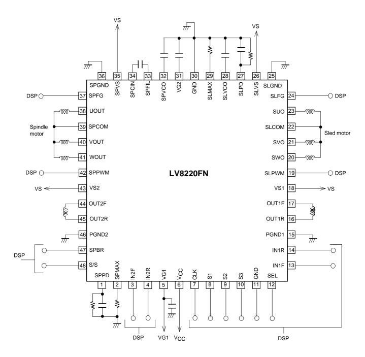
Insert a capacitor between VS and PGND and between V<sub>CC</sub> and GND.
