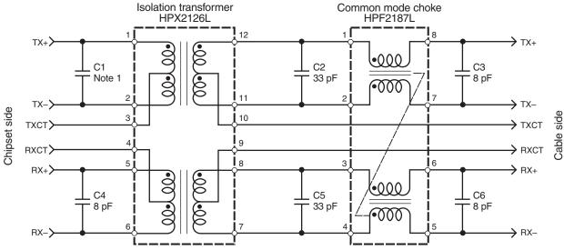
Note 1. C1 = 8 pF minus the output capacitance of the chipset
