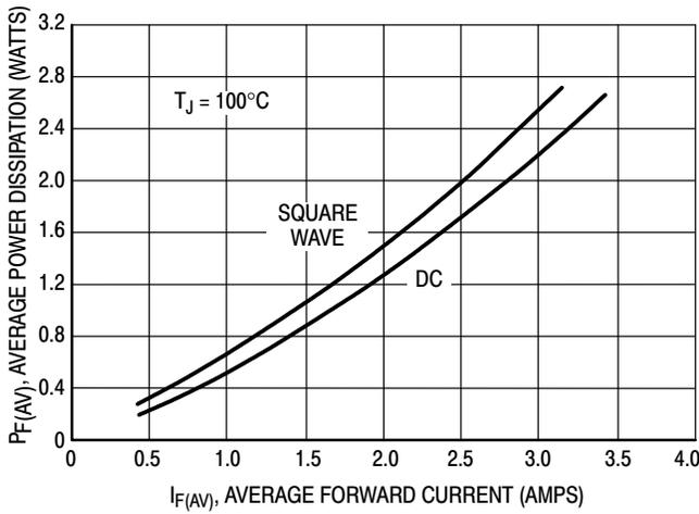
Figure 3. Power Dissipation
