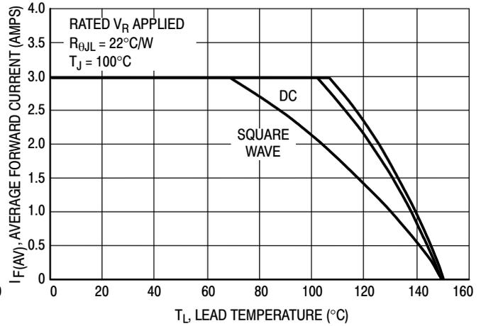
Figure 4. Current Derating, Lead
