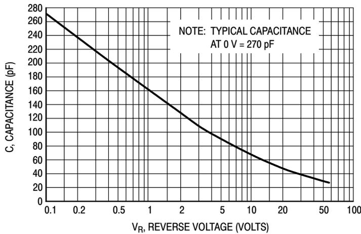
Figure 5. Typical Capacitance
