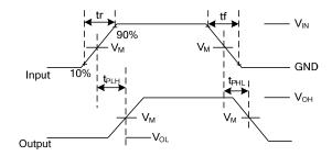
Notes: 1. V<sub>OL</sub> and V<sub>OH</sub> are typical output drop that occur with the output load.
