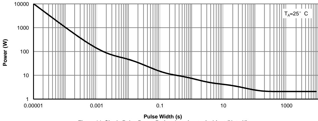
Figure 14: Single Pulse Power Rating Junction-to-Ambient (Note H)
