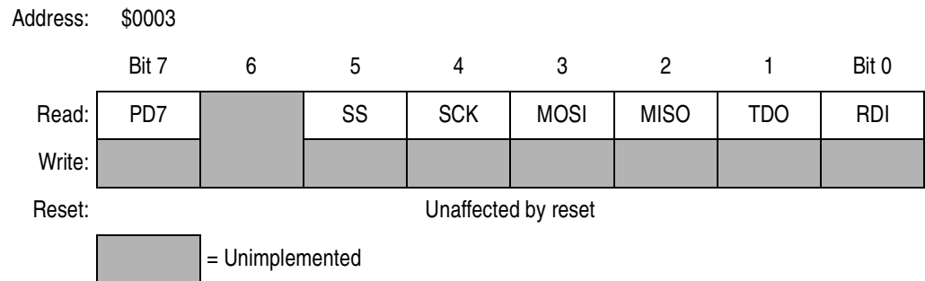
Figure 7-10. Port D Fixed Input Register (PORTD)
