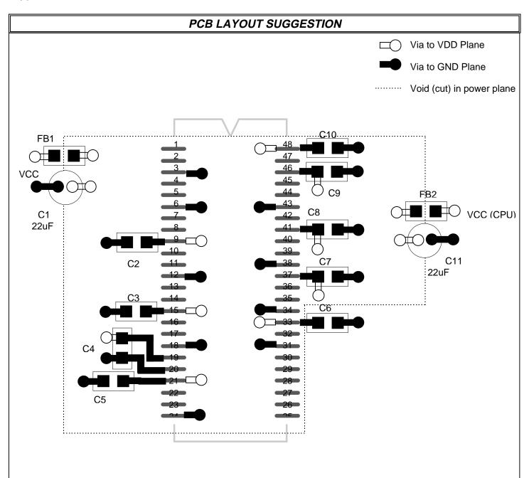
This is only a layout recommendation for best performance and lower EMI. the designer may choose a different approach but C2, C3, C4, C5, C6, C7, C8, C9, and C10 (all are 0.1 uf) should always be used and placed as close to their VDD pins as is physically possible. The topological hookup of C4 with respect to its power and ground vias is especially important.
