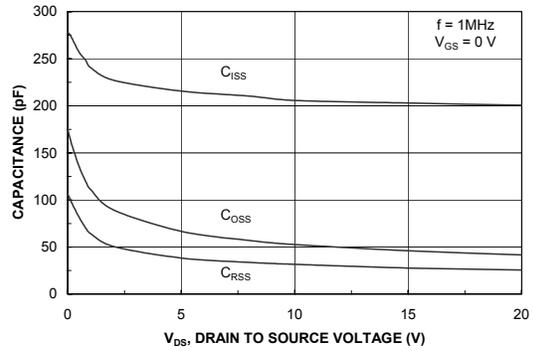
Figure 8. Capacitance Characteristics.
