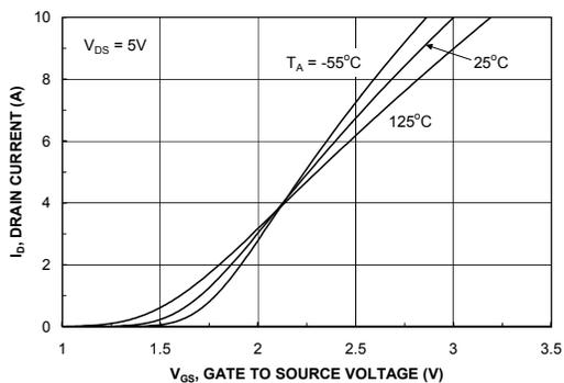
Figure 5. Transfer Characteristics.
