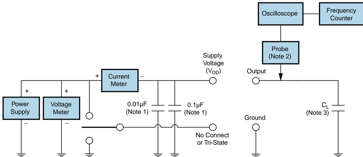
Note 1: An external 0.1µF low frequency tantalum bypass capacitor in parallel with a 0.01µF high frequency ceramic bypass capacitor close to the package ground and  $V_{DD}$  pin is required.
