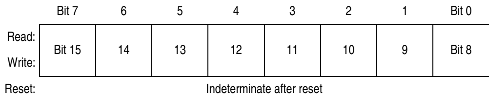
Figure 22-14. TIM Channel 1 Register High (TCH1H)
