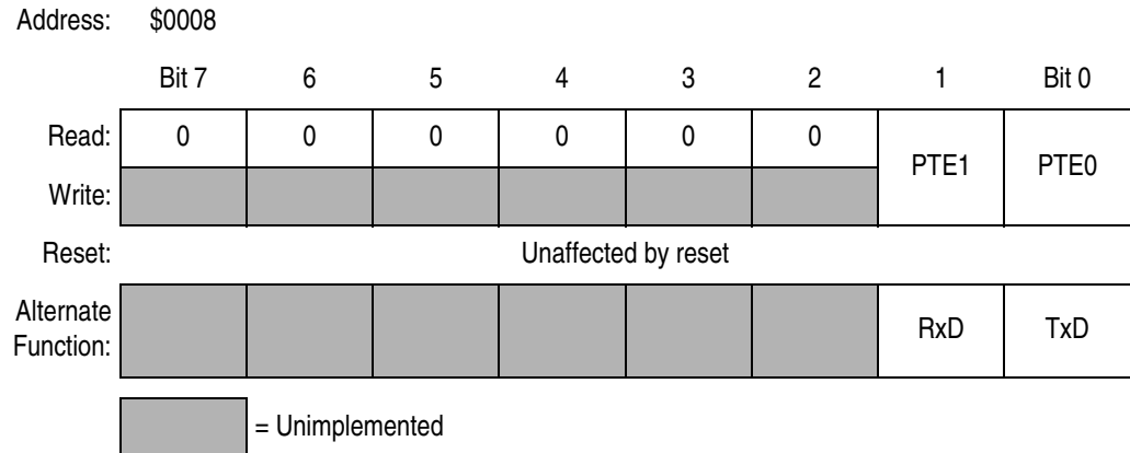
Figure 16-17. Port E Data Register (PTE)
